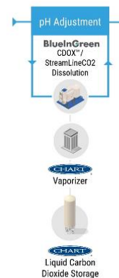
Figure 1. Common uses of CO 2 for pH Adjustment in Water Treatment. (1) Lime Softening – the process of adding lime (calcium hydroxide) to water to raise the pH and precipitate mineral (Ca, Mg) out of solution, after which, the pH is normalized by adding dissolved carbon dioxide, often called “recarbonation.” (2) Remineralization – the process of optimizing the mineral balance of water by simultaneously adding lime, caustic, or limestone with dissolved carbon dioxide to protect downstream infrastructure from otherwise aggressive water (such as RO permeate). The process increases alkalinity and is also commonly referred to as alkalinity adjustment, stabilization, or corrosion control. (3) Strong Acid Replacement – used in industrial wastewater pretreatment
