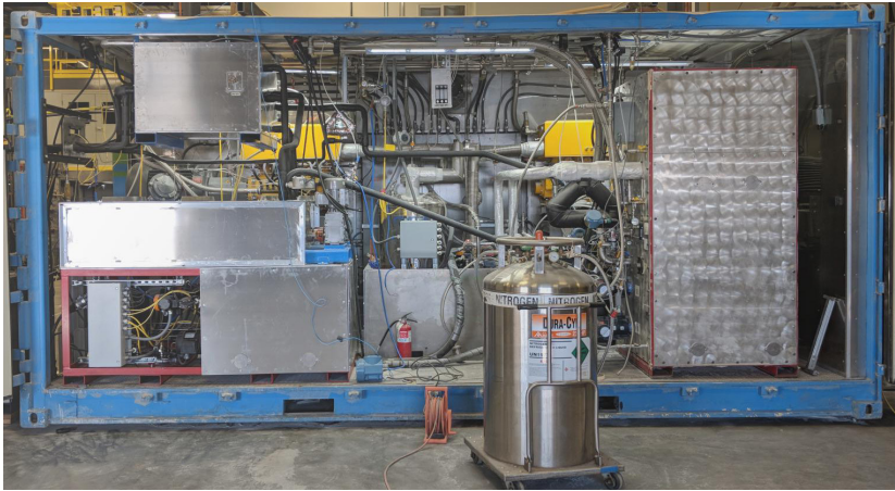
© SES | Cryogenic Carbon Capture small pilot as tested in the field
