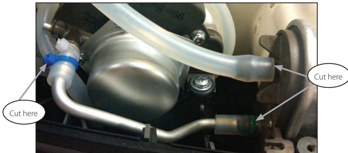
Figure 49: Cut Cable Ties
