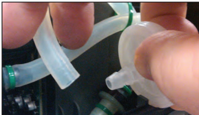
Figure 20: Disconnecting the HEPA Filter.
