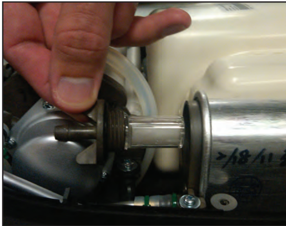
Figure 24: Unscrewing the HEPA Filter.
