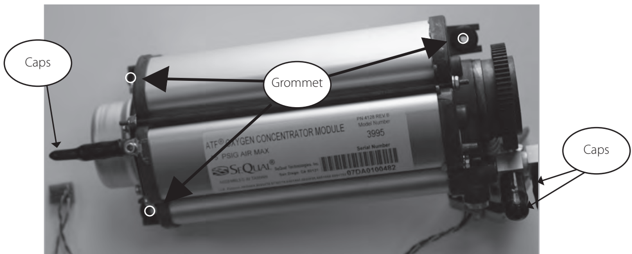
Figure 38: ATF Module Grommet Installation
