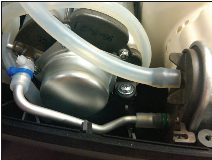
Figure 46: Product tank and hose barbs
