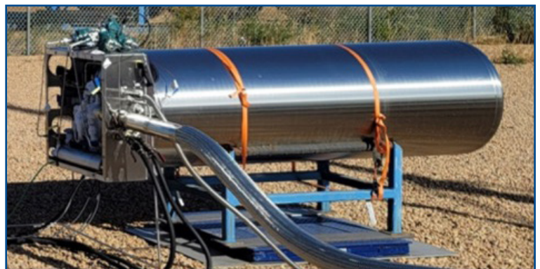
Testing Chart's onboard liquid hydrogen vehicle fuel system (HLH2) with fuel cell at our New Prague, MN (USA) hydrogen test facility.
