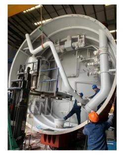
**Application:** Two new build chemical tanker vessels, of 28,000m³ each, built in China. The two tankers are fueled by Liquefied Natural Gas (LNG). Each ship carries 600m³ of LNG bunker fuel storage in two IMO Type C Tanks, designed to IGF Code. The ships being built by Wuhu Shipyard of China. M/T Prospero is the first of these two ships. Her sister ship is Pacifico, delivery June 2022.
