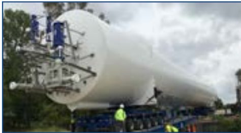
Largest Shop Built LH 2 Tank
