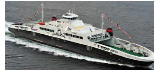
Noregian Fjord Ferries fleet uses two 125m 3 tanks with fuel supply system. Each Ferry carries 589 passengers and 212 cars.
