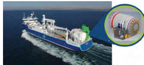
On Deck LNG Fuel Gas System with 135m 3 capacity. DNV Class Approvals.
