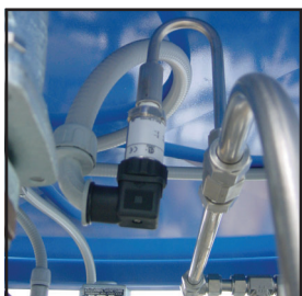
Integrated Bulk Tank Pressure Sensor
