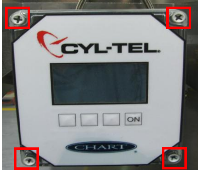
Figure 3.1.2-7: Red boxes indicate the 4 plastic screws that need to be unscrewed.
