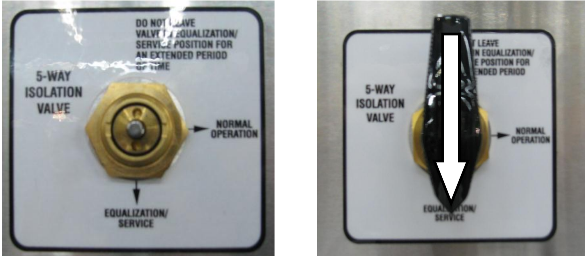
Figure 3.1.3-4: A) Use the nut on the 5-way valve to secure it to the tank. B) After the 5-way valve is secured to the tank place the black plastic knob back onto it.
