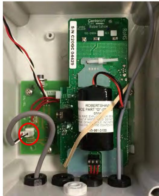
5. Plug the battery wire into the mating connector next to the battery.
