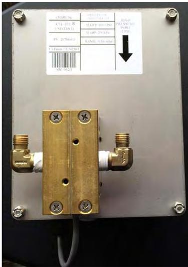
**Figure 1 - Elbows installed on the high/low sides of the DP sensor**
