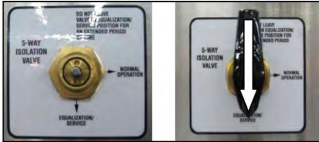
**Figure 11 - Use the nut on the Cyl-Tel isolation valve to secure it to the tank (left). After the Cyl-Tel isolation valve is secured to the tank place the black plastic knob back onto it (right).**
