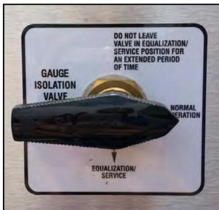
**Figure 5 - Cyl-Tel isolation valve in the Normal Operation position**
