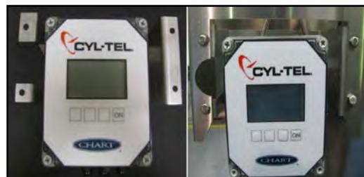
**Figure 10 - Cyl-Tel mounted onto the tank using the bulk mounting bracket**
