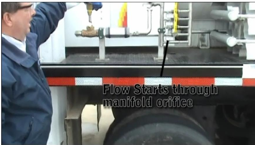
Figure 35 – Flow starts through manifold orifice
