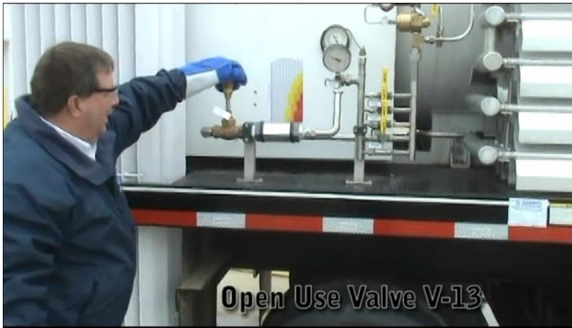
Figure 35 – Flow starts through manifold orifice
