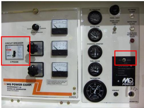
Located on the Road-Side of the MQ WhisperWatt is a control panel. When operating, the Circuit breaker must be ON, and the mode switch must be in AUTO.
