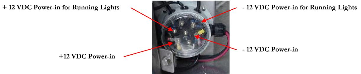
8. Is there power to the FlowcomS8? Use a Voltmeter to check the 12 VDC Power-in to the FlowcomS8 at the Main Board Terminal Strip X6. The Main Board is located at the rear of FlowcomS8 Stainless Steel Enclosure (see picture below).
