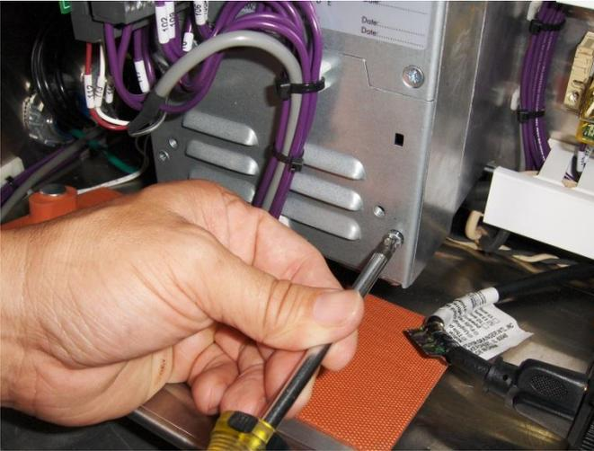
Remove the small panel on the lower front of the VFD by removing the two screws as shown.
