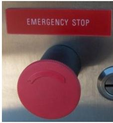
The Emergency Stop or “E-Stop” is located on the front of the control panel and provides an immediate way to stop the system from operating in the event should an emergency occur. When the Red Plunger is depressed, the system power will be shut off and all Air operated Valves will close. To de-activate the E-Stop button, turn the red plunger to the right until the plunger moves out.
