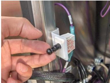
Whenever it is necessary for the Technician to have the system powered up with the Control Box door open, the Door Interlock Switch must be pulled out. Gently pull out the center pin as shown to over-ride this switch.
