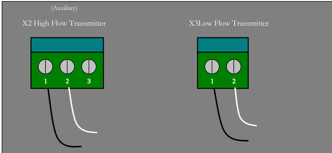
Above is a detailed view of X2 (Auxiliary) and X3 Low Flow Transmitter terminal blocks in the FlowcomS8. Using a Voltmeter and measuring across 1 and 2 of Block X2 or X3 should give a voltage reading of 24 Volts DC.
