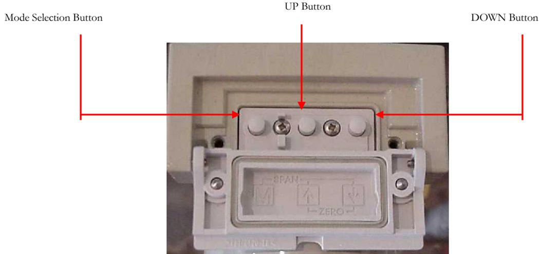
While the standard Orca System uses one Differential Pressure transmitter in its Metering system, a second transmitter is required for Dual flow Systems. It is also important to note that the D.P. Transmitters on your Orca system may not be interchangeable with each other. Systems with One Meter Section and Dual dispense capability utilize Transmitters with different internal spans. If you have questions regarding your system, call a Chart Representative for assistance at **1-800-400-4683**.
