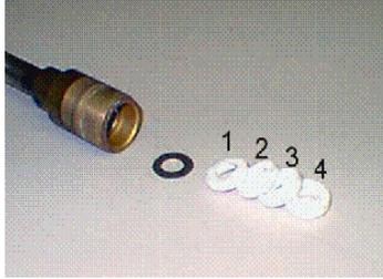
Remove Teflon packing rings (note washer if it comes out), carefully use a screw driver if necessary. When replacing the Teflon rings, make sure to put them back in order such that the one ring with the flat back (no. 1 in figure) goes in first. This one must go against the washer. Simply reverse the steps to re-assemble.
