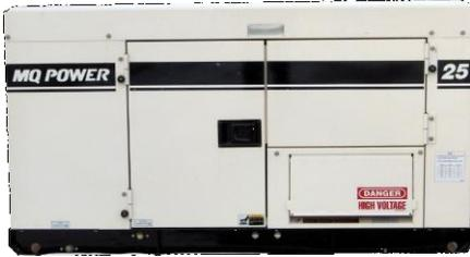
The DCA-25SSIU sports 27kVA/22kW standby output and 25kVA/20kW prime output. The generator is powered by a 4-cylinder, 31-horsepower Isuzu C240 diesel engine and the unit controls voltage regulation to +/-1 percent no load to full load. Sound level is an impressive 65dBA full load at 23 feet while the generator has a 17-gallon (65 liters) fuel tank.
