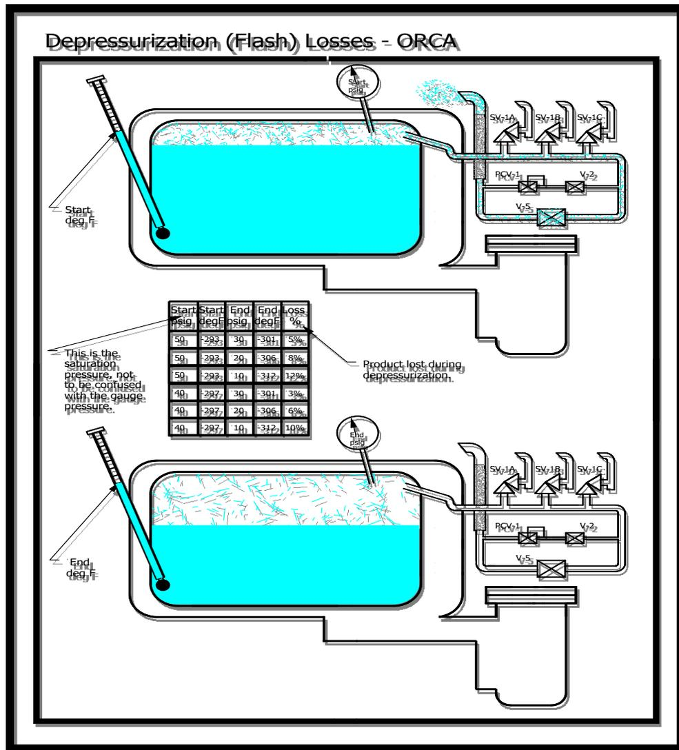
**Figure 10 - Flash Losses Bulk Storage**
