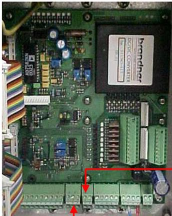
Left shows the wiring location of the Differential Pressure Transmitters inside of the FlowcomS8. For Troubleshooting the D.P. Transmitter, see section 6 of this manual. Electrical Schematics for the Orca system can be found at the rear of this manual.
