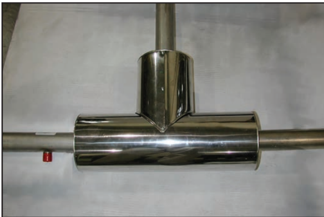
12. After completion, T-joint should look like this.
