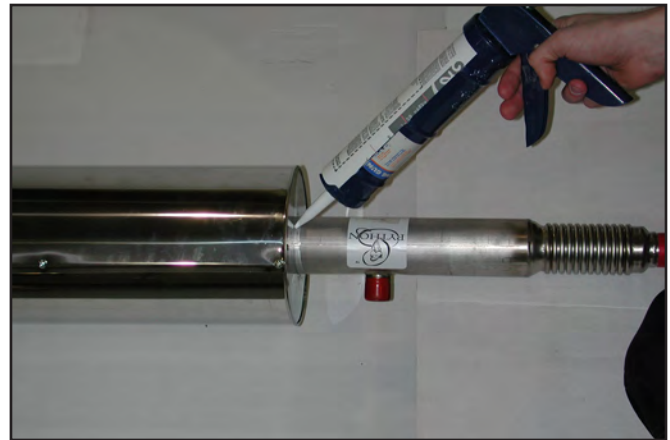
10. Caulk all edges with silicone sealer. (Sides and seams where metal cover overlaps itself.)
