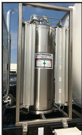
**High-Pressure Delivery Assist Option** – Capacity of 3300 scf in nitrogen service, delivery pressure up to 475 psig and flow up to 1800 scfh.
