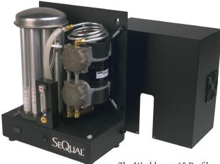
The Workhorse-23 Profile is a revolutionary oxygen concentrator system that provides 23 SCFH (11 LPM) of oxygen (including an oil-less compressor onboard) in the same space as the previous generation conventional two-bed 12 and 15 SCFH (6 and 7 LPM) systems.
