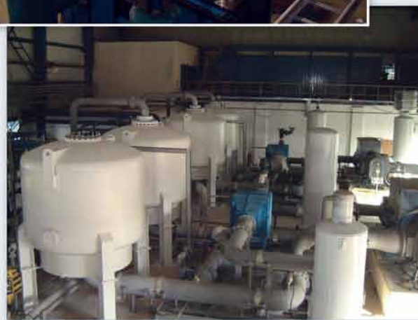
Gold Mine in Kazakhstan Two ASV33000 (868 Nm 3 /hr) Plants
