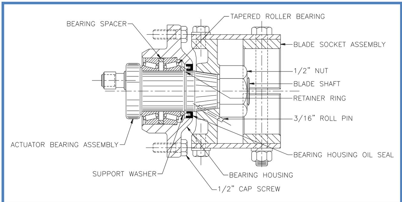
**Blade Socket/Bearing Housing Assembly**
