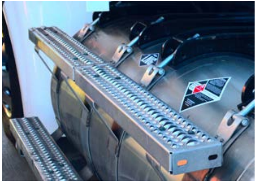
© Chart | Chart's vacuum-insulated fuel tanks for LNG are used by the trucking industry. LNG as an alternative fuel to diesel reduces the GHG emissions of ground transportation – an estimated $750m growth opportunity for Chart Industries
