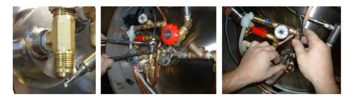
4. Loosen the feed through cable stainless steel fitting at the top of the feed through tee and pull out the cable from the tee as shown above. Discard old Flaretite seals. The tee <u>does not</u> need to be removed from the knuckle for cable replacement.
