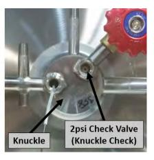
Locate the knuckle check in the port where the elbow was just removed. Note the positioning of the tabs in the knuckle check face. Align the tabs on the removal tool to match the knuckle check and insure they are fully engaged before trying to loosen.
