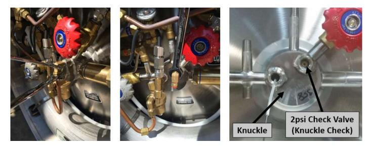
Locate the knuckle check in the port where the elbow was just removed. Note the positioning of the tabs in the knuckle check face. Align the tabs on the removal tool to match the knuckle check and insure they are fully engaged before trying to loosen.
