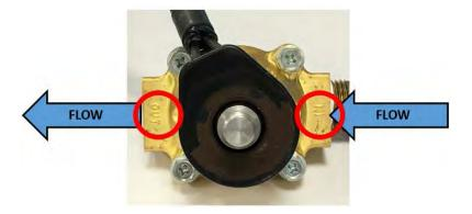
The solenoid "IN" connection will attach to the heat exchanger "OUT" line from the heat exchanger as seen below. The "IN" & "OUT" for the heat exchanger and solenoid connections are shown below:
