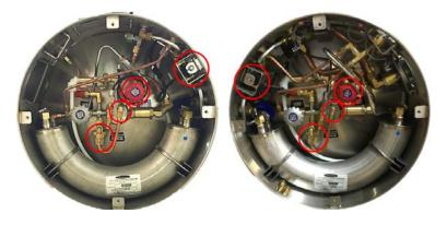
Excess Flow – In the event of a damaged fuel line downstream of the heat exchanger, Chart uses an excess flow valve on standard tanks and a normally closed electric shut-off solenoid on integrated tanks. The tank may have one device or the other, depending on the model of tank. They are used to shut off the flow of fuel in the event of an accident or damaged fuel line downstream of the heat exchanger.
