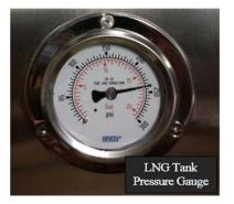
Note: If high tank pressures are present (above primary PRV set-point), determine the primary cause of increased pressure and repair before returning the truck to service.
