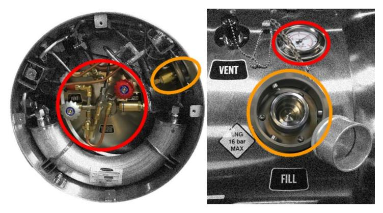
De-fueling is <u>REQUIRED</u> for all component and plumbing repairs within the <u>RED</u> circled areas.
