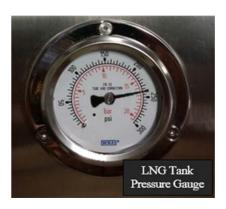
**Note:** If high tank pressures are present (above PRV set-point), determine primary cause of increased pressure and repair before returning truck to service.
