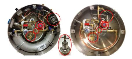
Excess Flow – In the event of a damaged fuel line after the heat exchanger, Chart uses an excess flow valve on standard tanks and a normally closed electric shut-off solenoid on integrated tanks to protect the heat exchanger from damage due to large flows of LNG.
