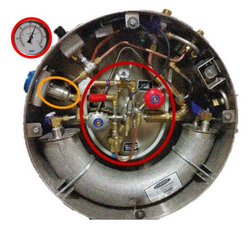
De-fueling is **REQUIRED** for all component and plumbing repairs within the **RED** circled areas.
