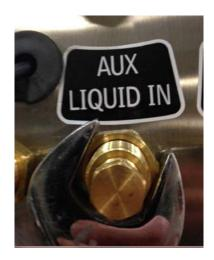
10. Remove the check valve, bulkhead connector, and 45° elbow fittings.
