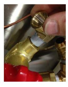
18. Reinstall 'AUX FILL' line using new ¾" Flaretite seals (remove old ones first). Tighten flare nuts with 1-1/4" combination wrench. If necessary, loosen jam nut of 'AUX FILL' bulkhead connector with 1-3/8" combination wrench to allow the tee going into the bulkhead connector to move to obtain proper alignment between tubes and fitting. Tighten flare nuts first and the jam nut of the bulkhead connector last.
