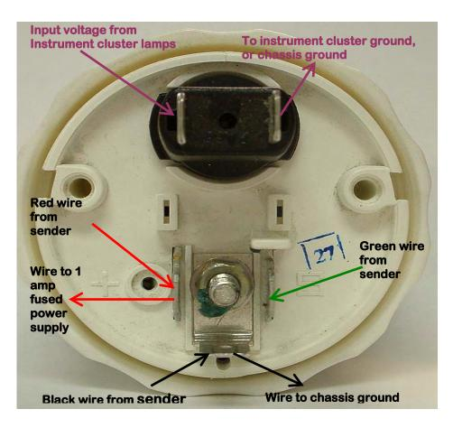
The three wires are to be connected to the following tabs on the back of the gauge.
