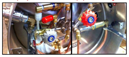
3. Use a 5/64" Allen socket and 7/16" box end wrench, loosen and remove the fill receptacle mounting bolts. Retain the mounting bolts and fill receptacle protective cap for re-use.
