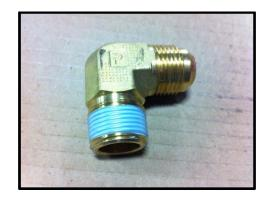
9. Mount the new receptacle in a vise and install the elbows male pipe threads into the receptacle threads. Tighten using a 1 1/16" wrench. The final stopping point should have the elbow flared outlet facing to match the orientation of the elbow on the original receptacle (orientation note from Step 6).
