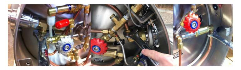
3. **Prior to removing receptacle, note the orientation of the elbow on the fuel receptacle.** Use a 5/32" Allen socket and 7/16" box end wrench, loosen and remove the fill receptacle mounting bolts. Retain the mounting bolts and fill receptacle protective cap for re-use.
