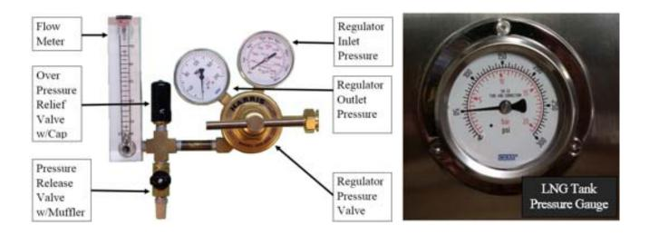
**Step 6:** Close the Pressure Release Valve on the tool, slowly open the Liquid Shutoff Valve (red handle) on the LNG tank, and turn the truck key to the "ON" position.
