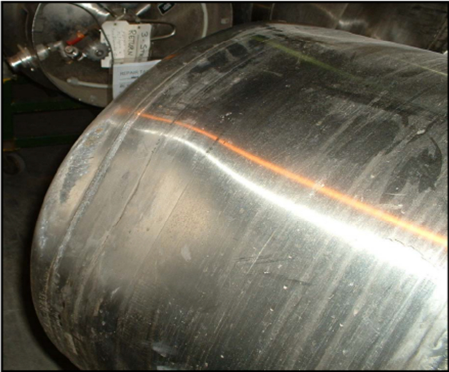
Photo 3 – Level II Damaged outer shell, rear head and welds
