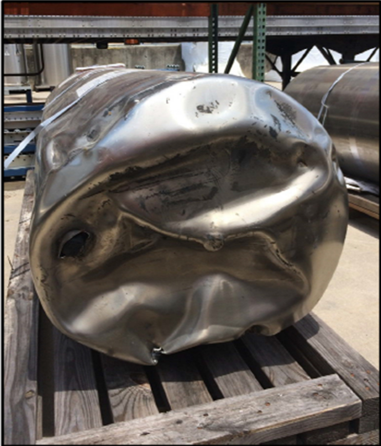
Photo 6 – Level III Extensive damage to outer shell, rear head and tank support
