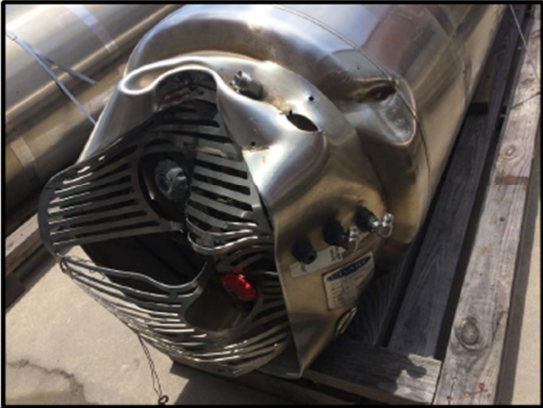
Photo 5 – Level III Extensive damage to shroud, front head and tank support
