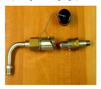
Set the nitrogen tanks supply regulator to 100 PSI/7 bars. Connect the female vent nozzle to the male vent receptacle (right side of photo above) on the tank. Open the control valve on the nitrogen source. Re-check the regulators pressure gauge to ensure the regulator is set at 100 PSI/7 bars.
