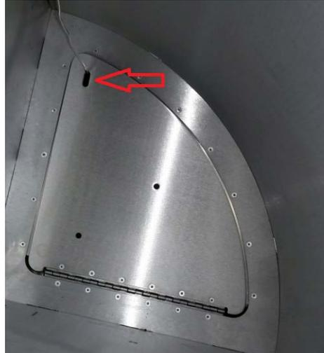
4. Lift the access panel until it is completely open.
