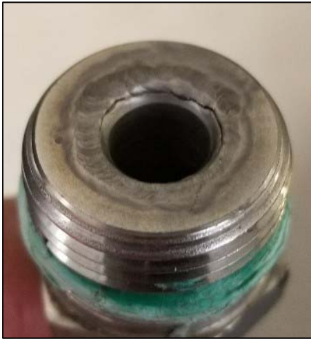
Chamfer in tube assembly defect
