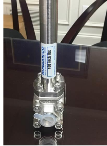
New style Habonim Valve with Duncan inspection sticker. p/n 21070662
