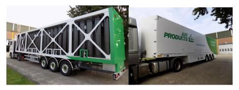
Today's state of the art solution for high pressure Hydrogen trailers is hitting the road in Europe. The unique design is due to European regulations covering trailers of this size. The 'inside the box' photo (above left) shows a system comprised of 135 interconnected, vertical, high pressure cylinders engineered and built by Chart's GOFA facility in Germany,
