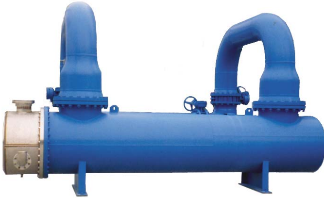
Thermax Inc. Model P300-30 CW rated at 3.5 million BTU's/Hr using 5,000 GPM, 55°F cooling tower water for oxygen vaporization.
