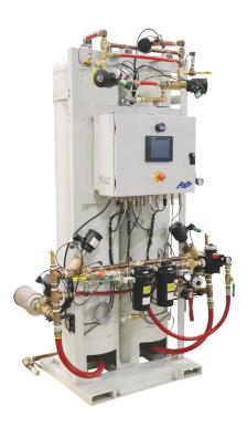
AirSep Alpha Series Nitrogen Generators produce from 450 to 44,671 cubic feet of nitrogen per hour at 99.5% nitrogen concentration. When electricity and an adequate source of compressed air is supplied, these dependable machines can provide nitrogen for practically any application and at concentrations up to 99.999% (10 PPM O2).
