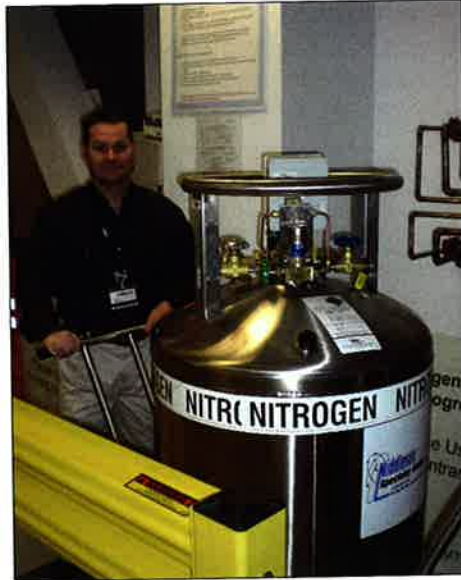
Tom Stack mounts a 230-liter nitrogen Perma-Cyl with Cyl-Tel gauge onto the scale of their Low-Loss fill station.
