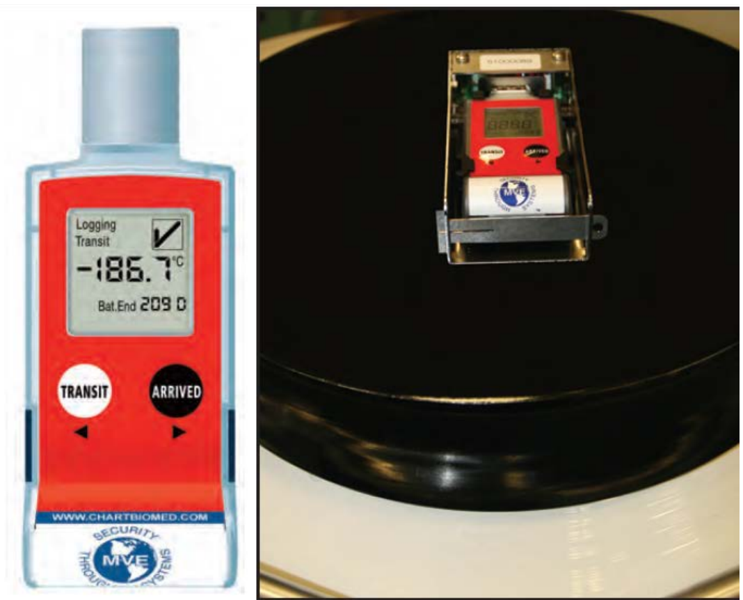
Fig. 1 - PDF Logger (left) and PDF Logger complete with bracket mounted to lid assembly (right)
