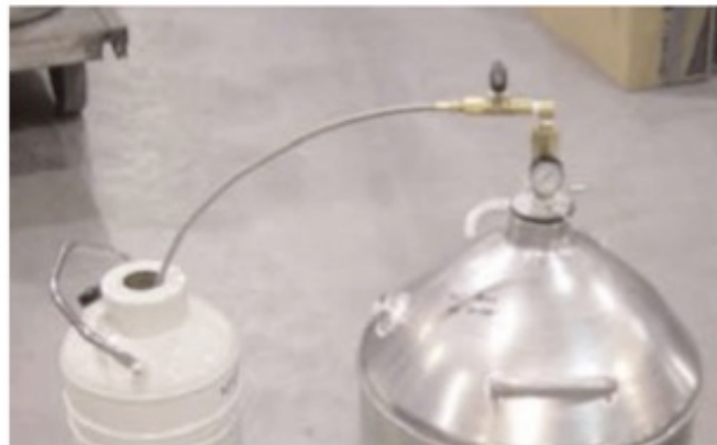
Stainless Steel Transfer Hose in Use
