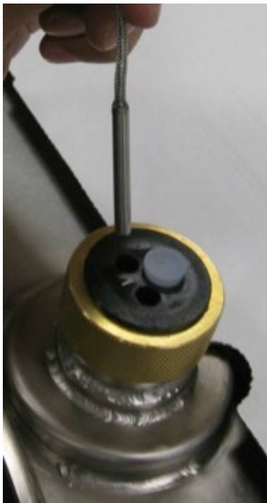
Temperature Probe Being Removed from a High-Efficiency Freezer
