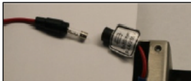
Figure 1 - Battery Backup Fuse
