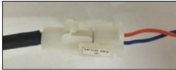
Figure 6 - Battery Backup Connector. Black - from the Battery Backup. Dark Blue/Orange - from the TEC 3000 Wiring Harness
