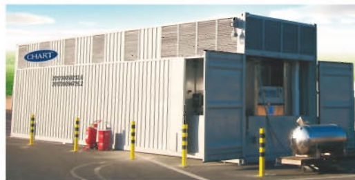
Movable LNG station in the 49 ft container, tank volume 30 m 3
