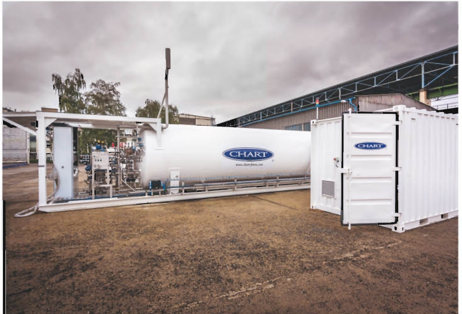
Movable LNG station with a submerged pump, saturation vaporizer, tank volume 31 m 3 to 60 m 3 , up to 160 truck fuelling charges
