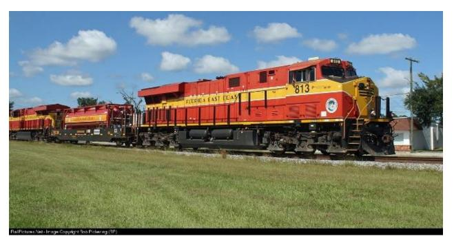
In 2016, Florida East Coast Railroad, converted its entire fleet of locomotives to dual fuel, replacing 80% of the diesel fuel with natural gas. Chart's contribution to the project was the design and manufacture of 13 LNG fuel tenders. In its popular Clean Cities series, Motorweek released a short video that highlights the environmental and economic benefits of this first-of-a-kind. *The video can be viewed here Florida East Coast Railway's LNG Trains*
