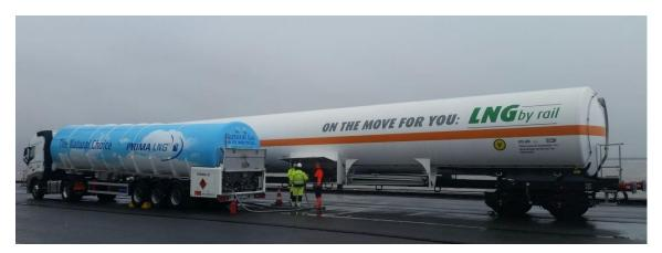
LNG has been approved for transport by rail in Canada since 2014. In Europe Chart and VTG teamed up to develop the LNG rail car pictured above. It has a capacity equivalent to two road trailers and is designed to transport LNG long distances and support high volume energy users, such as gas fired power stations.
