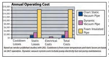
vacuum pump installed with the pipe system that continuously pumps on the annular space to maintain a vacuum. Dynamic vacuum systems are significantly more efficient than foam insulated systems; however, they have significant operating cost and reliability issues. Static vacuum insulated systems are the most thermally efficient and have the lowest operating costs.
