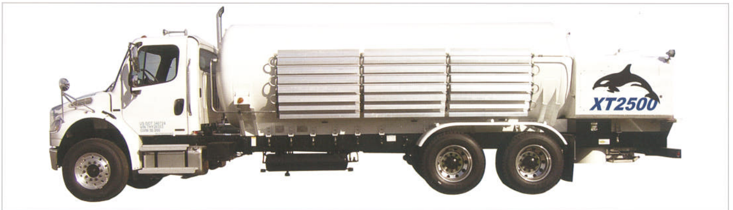
The ORCA XT2500 is designed so liquid can be quickly dispensed from larger horizontal vessels. Photo courtesy of Chart Industries.
