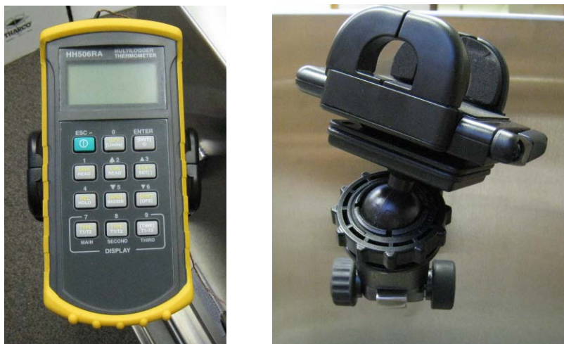
Figure 2b - Mounted Thermometer and Adjustment Socket (Model PN 14448703 only)
