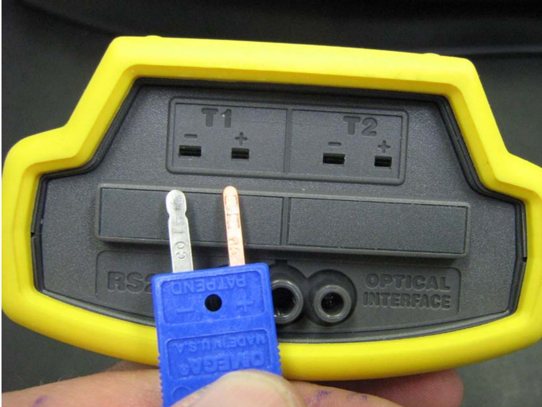
Figure 2c - Installation of thermocouple into thermometer (match +/-)
