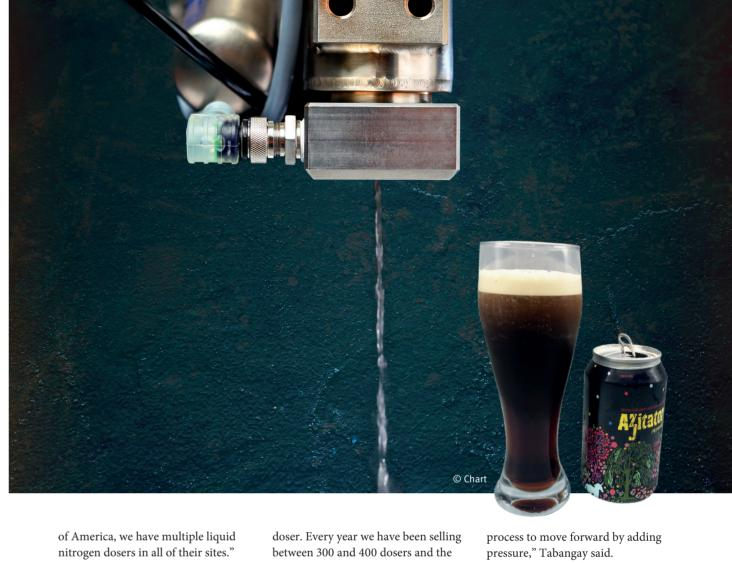
applications, the rapidly expanding gas is allowed to escape before the product is sealed, flushing out oxygen, and extending product shelf life. According to Chart, "documented studies show a 26% increase in shelf life and 95 to 98% reduction in headspace oxygen compared to traditional gaseous nitrogen purging". The US-based cryogenic equipment manufacturer also claims that there is a "46% reduction in nitrogen consumption using a Chart doser in lieu of traditional nitrogen gas purging".
