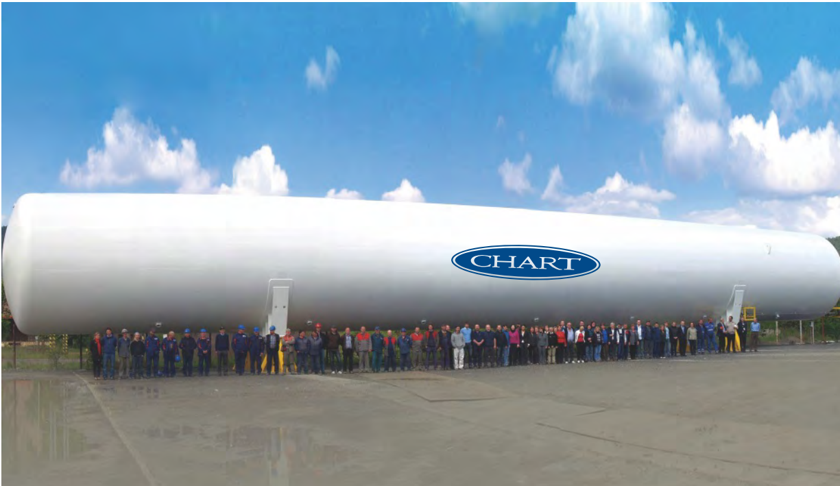
Construction of the 1000 m³ large-scale storage tank for the Norwegian project (made in the Czech factory)
